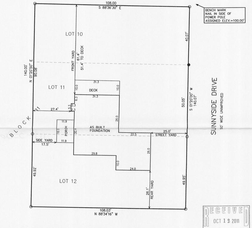
LOWEST GROUND ELEVATION AT BUILDING FOOTPRINT=100.8' PLUS 35' MAXIMUM BUILDING HEIGHT MAXIMUM ROOF PEAK ELEVATION=135.8 AS BUILT PEAK EL. = 128.7'
